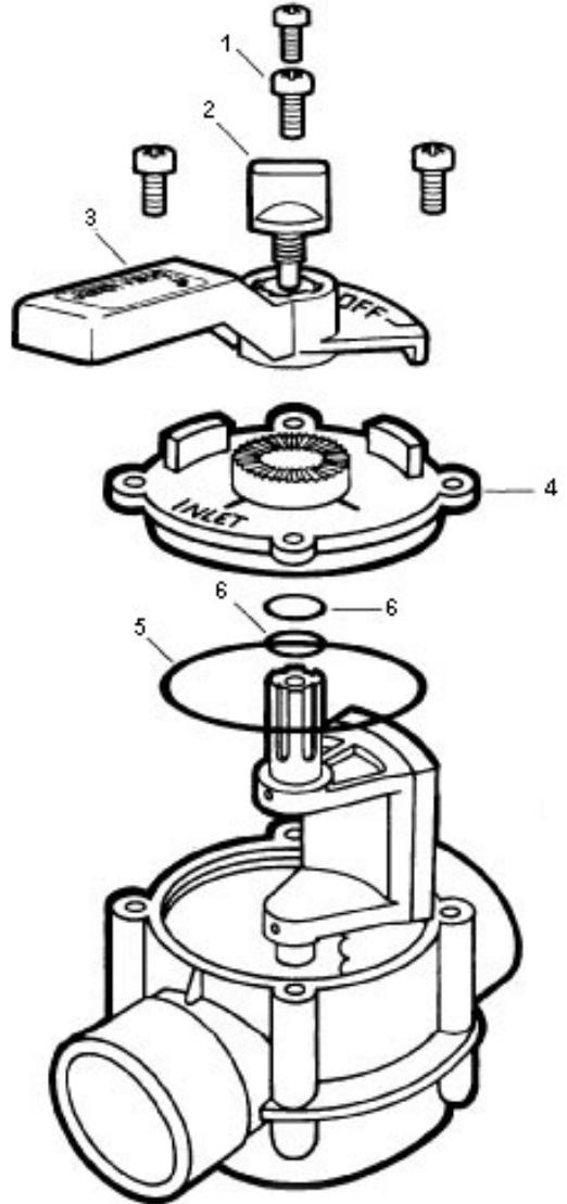
**NOTE** The valve housing is not available as a separate part. To replace the housing, you need to replace the entire valve.
